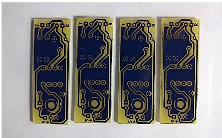
The PCB's after etching.
