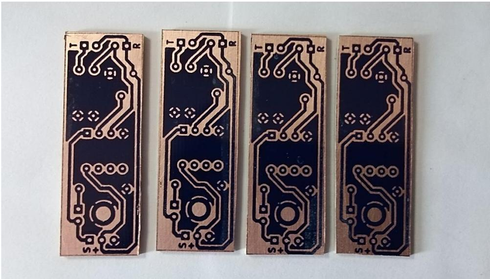
The PCB cut and ready for etching.
