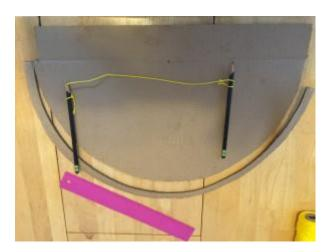
Once all of your long pieces are shaped, you can begin assembling the antenna. At this point it begins to be putting pieces of the puzzle together with one exception. You must bend the long pieces on their perpendicular axis. This can be a bit tricky, so here is how I did it.
