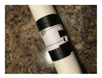
Lastly, you will need to drill holes for the coax balun. This can be done anywhere on the pipe, but I did it about 6 inches below the top holes. Take your coax and wrap it around the pipe so the end result will be 4 complete turns and mark where the coax will go through. After this step you might want to consider painting the PVC pipe. I will generally use a fine sandpaper then spray paint it with
