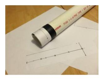
Next you will do almost the same again, this time you will cut a 50mm wide strip of paper. Make two parallel lines on the paper exactly 24mm apart. Take your measurement (Circumference divided by 4) and mark your drill points on the paper, this time staggering the points between the two lines.
