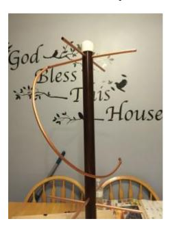
Grasp the top connection with one hand and gently bend the 812mm piece to meet the lower cross bar on the opposite size. You must bend the ENTIRE antenna ANTI-CLOCKWISE when viewed from the top. I repeat, you must bend each leg ANTI-CLOCKWISE. The bend should be as even as possible, and I frankly don't have any magic way to get this done or confirm it was done correctly other than the old hairy eyeball.
