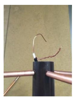
Then strip the piece of coax so that you have a few inches of extra center conductor and shield like in the picture above. Wrap the center conductor around one of the wires you stripped earlier and solder it, then wrap it in tape. I placed a piece of rigid foam on the inside so that the copper pieces won't touch and subsequently short out the antenna after final assembly. When this step is finished, your mess should look something like this:
