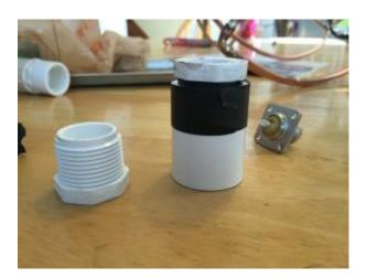
My antenna has been up for over a year now, and this solution worked. It appears as if there are no leaks and it still functions properly. Mounting this antenna is another animal that will be left up to your situation. I ended up taking a  $1 \frac{1}{4}$ " to  $1 \frac{1}{2}$ " coupling and mounted the antenna on top of a piece of 10ft,  $1 \frac{1}{2}$ " pipe.
