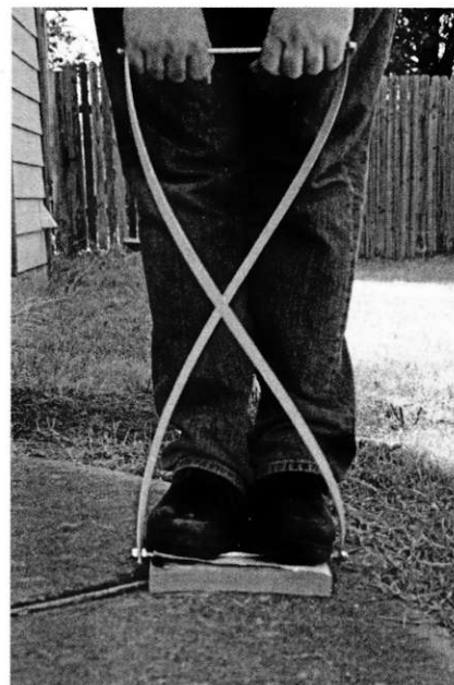
Figure 3 — Hold one aluminum rod end of the rectangle in your hands while standing on the other end on top of the book, and twist the rectangle to the right while pushing down.
